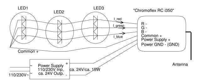
The example above uses 3 LEDs. A 4 wire cable is used, where 1 wire is a simple pass-through for the common +.
